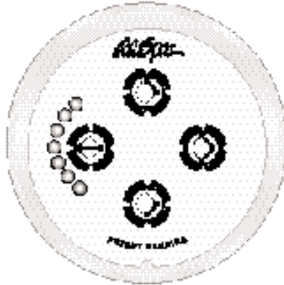
Figure 10. Cal Spas Flow Diverter
